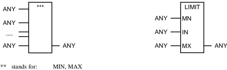
Figure A.7. Graphical declarations of the selection functions MAX, MIN and LIMIT
