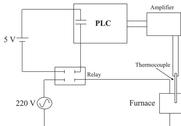
Fig. 1 A temperature control system of a resistive electric furnace.
