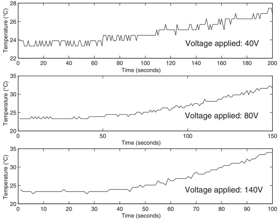
Fig. 5 Time delay of the furnace step responses.
