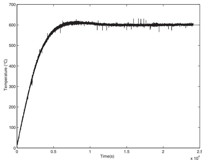
Fig. 11 Step responses of the compensated feedback system.
