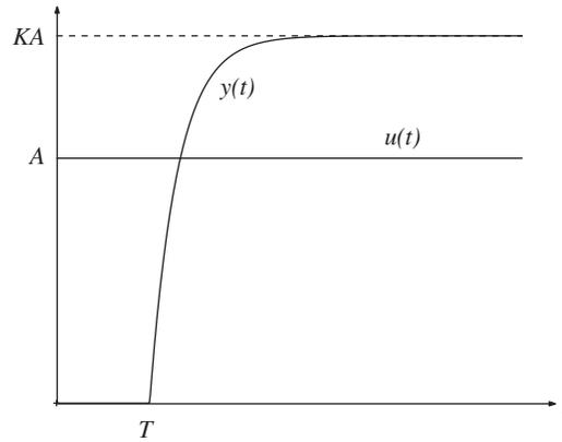
Fig. 2 Step response of a stable first order system with time delay.
