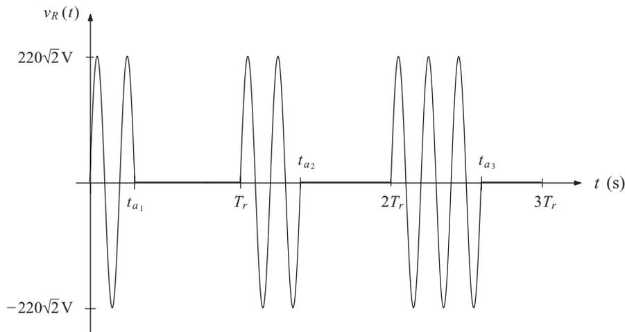
Fig. 10 Typical curve of a solid state relay.
