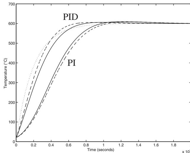
Fig. 9 Reaction curve and simulated step responses of the compensated system.
