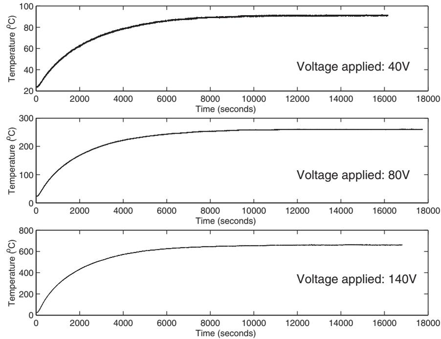
Fig. 4 Furnace responses to sinusoidal voltages.
